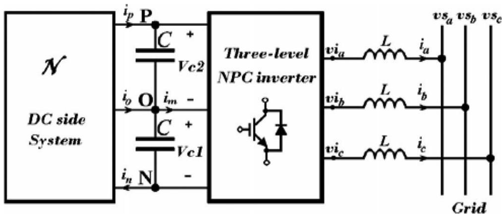
Fig. 2. General diagram of a grid connected three-wire three-level inverter
