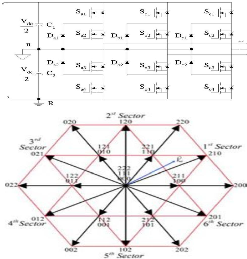
Fig. 1. Typical three-level inverter (a) structure of circuit, and (b) three-level Inverter space vector diagram for balanced dc-link capacitors
