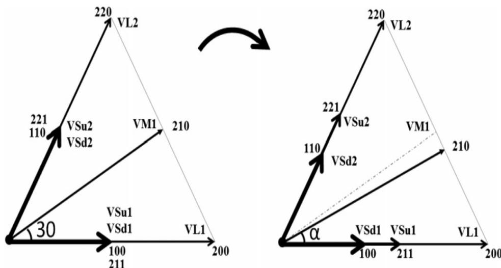
Fig. 3. Vector diagram in the first sector of Fig. 1(b) showing the change of the vectors using balanced dc and unbalanced dc assuming  $V_{c1} < V_{c2}$
